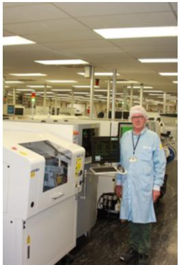
a special line for the production of ceramic boards which are part of components for an automotive tier 1 supplier. Since the JUKI GL printer comes with all necessary appliances for vacuum fixing of the circuit boards, a customer specific fixture could be installed quickly and easily. The printer has also been audited very closely by the customer on its attributes.
