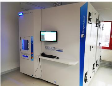
Thanks to the design of the automated storage cabinet combinations, Lacon benefits from storage space for more than 4000 component reels. What is more, the ISM500 offers 400 storage places for varying component containers, in this case primarily for sticks and/or bagged component segments. By relocating the SMD components into the ISM system, it was possible to remove an existing high-bay rack of more than 10m in length. The freed-up space can now be used for other production units.
