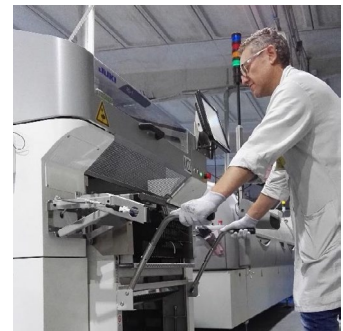
Upon positioning of the feeder bank, each feeder position is automatically recognised. (Image: NES)
