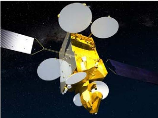
These terminals are able to communicate data and pictures via laser beams between the satellites, and from the satellites to Earth. Benefits of the laser communication are, for example, the high digit rate of currently 5,5 Gbit (this equates to 200.000 DIN A4 pages) per second and their insensitiveness to disturbance.
